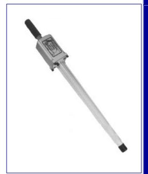
The model GA-72Cd Magnetic Locator detects the magnetic field of ferromagnetic objects. It responds to the difference in the magnetic field between two sensors, which are spaced about 14 inches apart.
